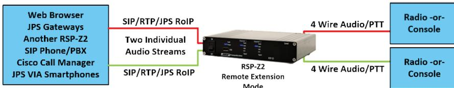
**Above:** The RSP-Z2 functioning as a pair of independent Radio to IP interfaces. There is a single RJ-45 Ethernet Port and IP address, but in the Independent Passthrough Mode, each path remains independent of the other. The transport protocol for each path (RoIP/SIP/RTP) is user-configurable, offering flexibility for varying system requirements.
